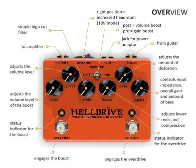
There are trimmer resistors inside the unit for BASS and PRESENCE (overdrive) and GAIN, BASS and TONE (boost). Simply unscrew the bottom plate and follow the instructions on the back.
